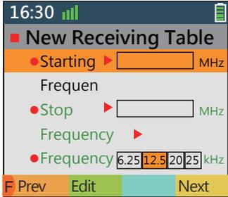
**8b** Use the 4-way button and Keypad to complete the input of each parameter on the screen, and then press Save.
